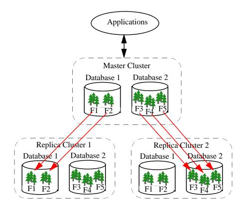
A cluster can contain both Master and Replica databases. On Cluster A in the example shown below, Database 1 is the Master database and Database 2 is the Replica database.
