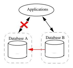
• Running a backup operation on Database B and restoring Database A from the backup file, as described in <u>Backing Up and Restoring a Database</u> in the *Administrator's Guide*.
