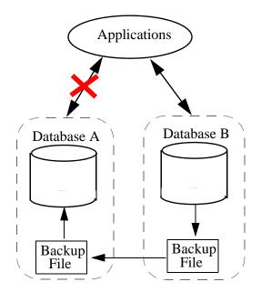
Once the data has been restored on the Database A, you can redirect the applications from Database B back to Database A.
